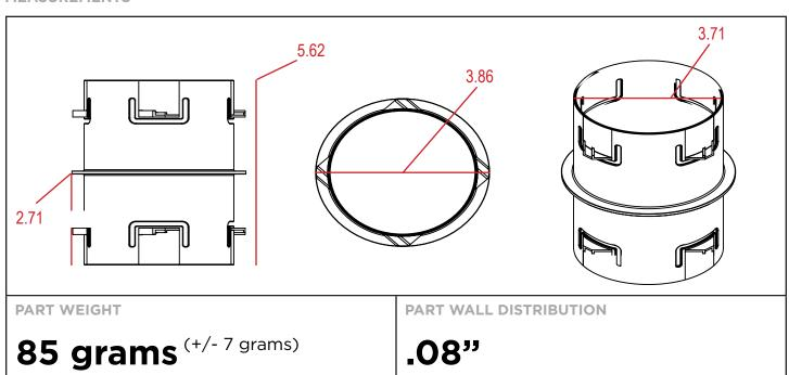
These specifications are held in standard according to ASTM F667 - Standard Specification for Polyethylene Plastics Pipe and Fittings material.
